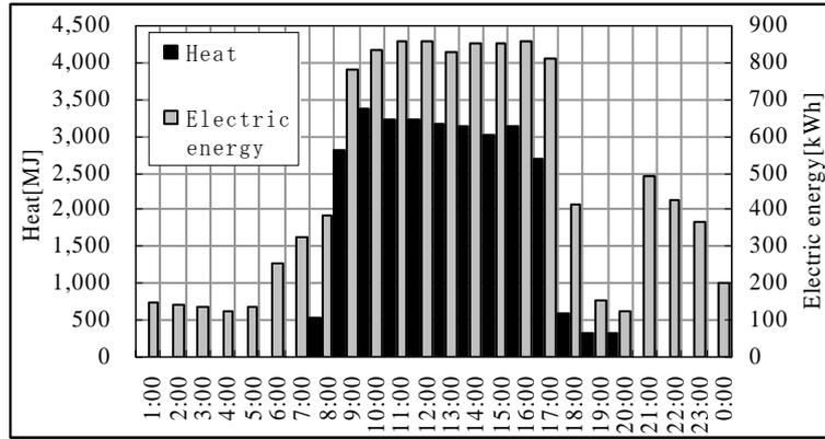
**Figure 2 The transition of the heat and the electric energy on the representative day of summer**
